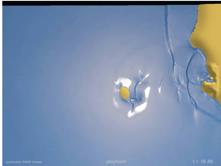
Figure 6: Complex reflection patterns and run-up into Monai Valley simulated by ANUGA and visualised using our netcdf OSG viewer.
